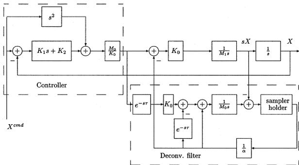
The dashed box marked “controller” produces the control input  $f_0$ , a feedback control, which is fed both to the system and, with one step delay, to the compensator (which is the dashed box marked “deconv. filter”).
