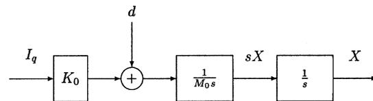
where  $M_0$  is the mass of the rotor,  $K_0$  is the thrust constant,  $X$  is the angle of the rotor,  $I_q$  the thrust current, and  $d$  represent disturbances entering into the system. For the sake of simplicity, we use the frequency domain notation.
