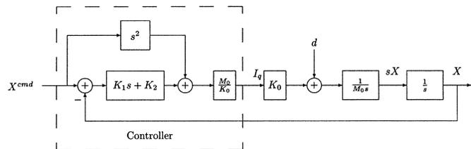
The signal  $X^{\text{cmd}}$  represents the path to be tracked by the output  $X$ . It is fed to the dashed box marked “Controller.” This is the acceleration controller, which produces the input fed to the system.
